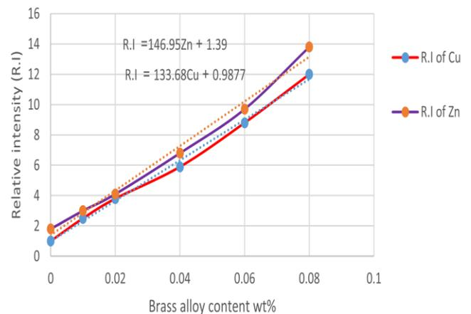
Figure 3: Calibration curves for brass alloys in organic liquid
