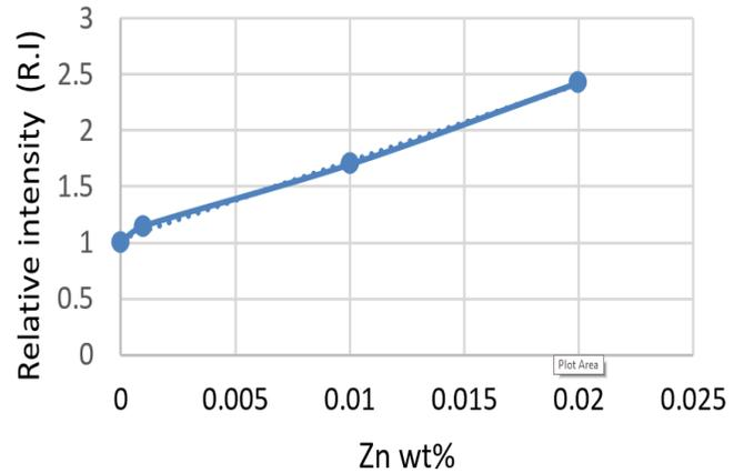
Figure 1 : Calibration curves for Zn suspended in oil
