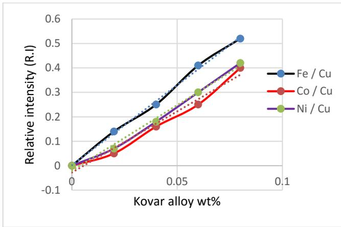
Figure 4: Calibration curves for Kovar alloys in organic liquid
