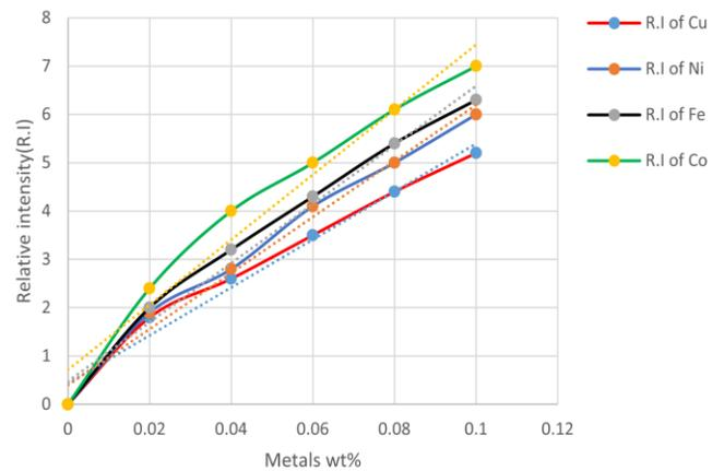
Figure 2: Calibration curves for pure metals in organic liquid
